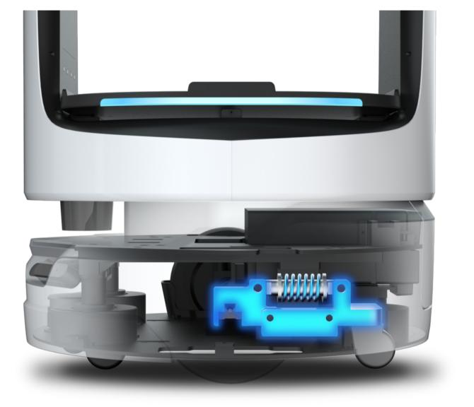
The newly developed interlinked suspension in automotive grade can adapt to surface undulation, effectively reduce the shake due to floor roughness and achieve excellent running ability.
