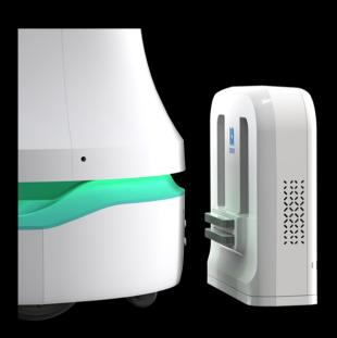
The total battery capacity is 51.2Ah, for a maximum disinfection time of up to 6h, which can support the disinfection of 12-15 rooms (20m²/room). Puductor 2 is equipped with a docking station. To make sure that the robot is fully charged and ready for the next task, timesaving as it requires no involvement from your staff.
